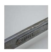
Discoloration from exposure to excessive heat.
